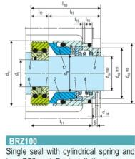
sleeve (Item no. 2) for use with guench. no. 1) either metal or silicon carbide. Insert (Item no. 1) either metal or silicon Optional without maintenance rinsing. carbide.
